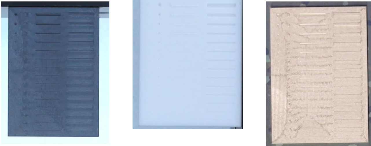
Figure 47: 3D resolution specimens with dark matt (Rescor ceramic), white translucent (Macor ceramic) and reflective metallic (Aluminium) surface
