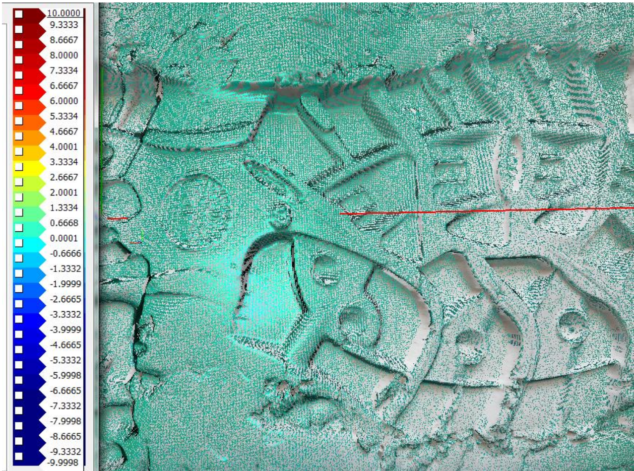
Figure 57: Differences analysis between the final mesh model and the point cloud. All the points are coloured cyan indicating they are within the tolerance.
