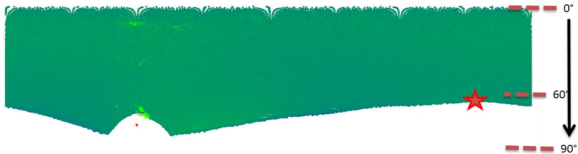
Figure 5: Enrolled view of the measured sphere in sphere coordinate system
