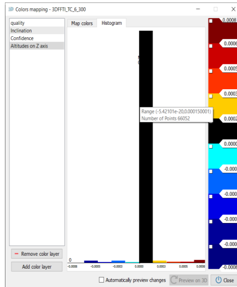
Figure 39: Histogram of the height colour map applied to the 6 simulated scans
